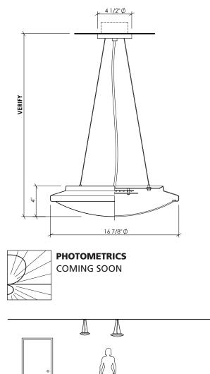
**MOUNTING:** Standard J-box or plaster ring. Safety cable provided.
