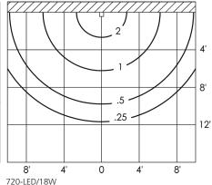
720-LED/18W 690 FIXTURE lumens 10' Mtg. Ht. Horizontal Illuminance at FF
